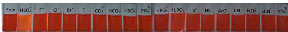
Fig. 1 a UV–vis absorption spectra of L (10.0 μM) with gradual addition of \text{HSO}_4^- [0, 2, 4, 6, 8 and 10 equiv., respectively] in THF–H 2 O (8/1, v/v); b Color changes of L ( 1 \times 10^{-4} M) upon addition of different anions in aqueous solution (THF/H 2 O=8/1, v/v)
